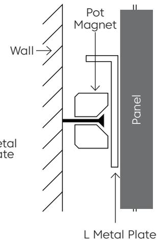
L Plate Wall + Metal Plate Configuration
