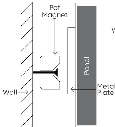
Wall Pot Magnet Install L Plate + Metal Plate
